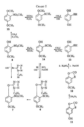
The structure of the methylation product 6 was also confirmed by reaction of 2-methylthio-4-methoxyphenol (14) with 5-bromo-1-phenyltetrazole (10).
